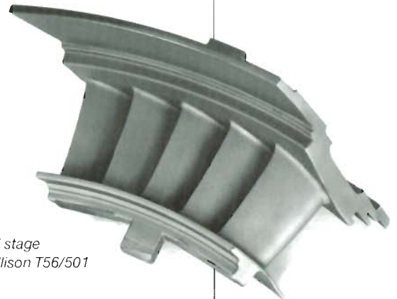
Second stage blade. Allison T56/501 engine with ACME masking boot.
