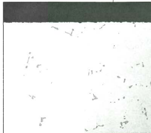
Shown above are the microstructures of a nickel base turbine component before and after AEP 32 coating.
